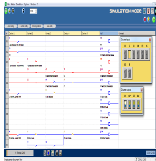
Gambar 4. Pengoperasian Motor Pompa Transfer
