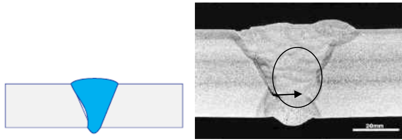
Gambar 12.15 lack of sidewall fusion (TWI, 2018)
