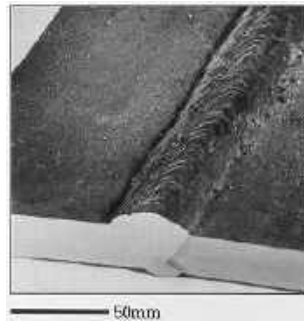
Gambar 12.26 excess weld metal (TWI, 2018)
