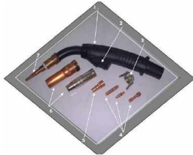
Gambar 5.4 komponen utama Torch; 1) Torch body, 2) On/off or latching switch, 3) Spot welding spacer attachment, 4) Contact tips, 5) Gas diffuser, 6) Gas shrouds dan 7) Torch head assembly (minus the shroud)
