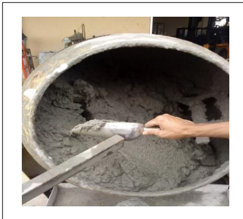
Gambar 3.3 Proses pencampuran mortar foamed concrete dan FCRHA
