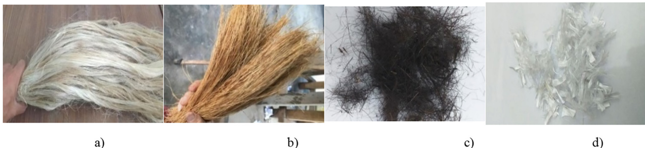
Fig. 1. The fibers used in the study: a) PALF, b) CF, c) ISPF, d) PPF
