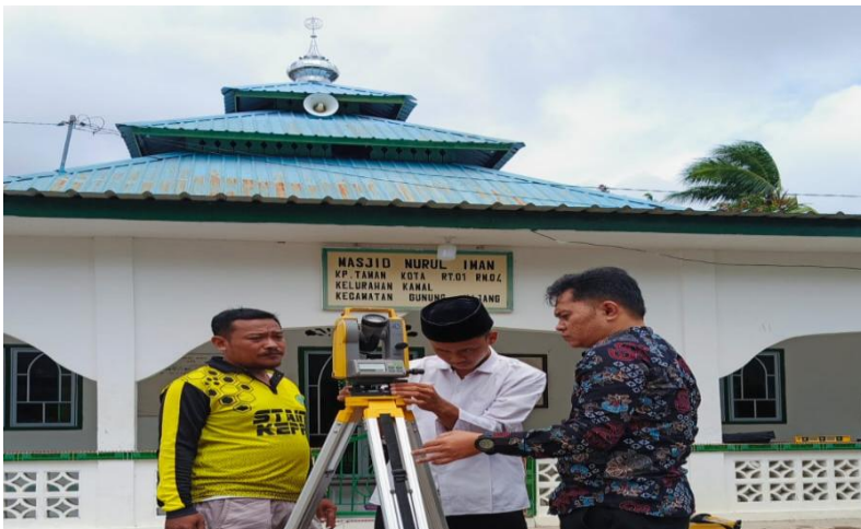
Figure 3. Determining the Solar Azimuth Using a Theodolite
